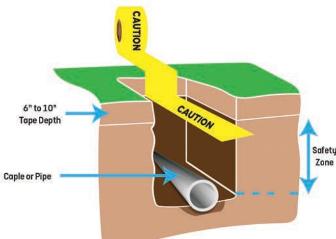
Underground warning tape is normally installed a specified distance directly above the service line so that any future excavators will be aware of the cable or pipeline further below.
